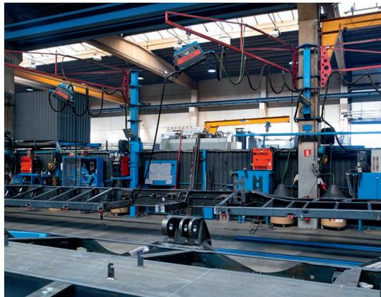
More than 160 MicorMIG 400 are working in the five plants of Faymonville Group. The MIG-MAG welding inverter scores with the SpeedArc process for a focused arc, high welding speed, and simple, multilingual operator guidance.
