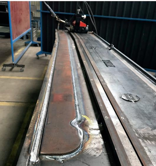
The welding tractor is quick to install with a simple device and produces rework-free uniform weld seams.
